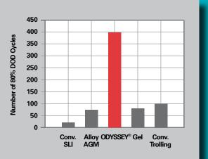
**Long Cycle Life** ODYSSEY<sup>®</sup> batteries routinely deliver up to 400 deep cycle (80%) discharges.
